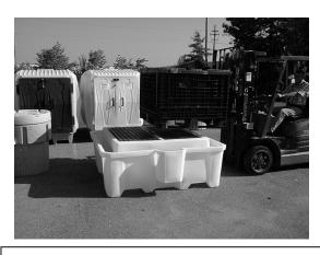
4.) Load the IBC container onto the pedestal of the IBC 2000i from the side.
