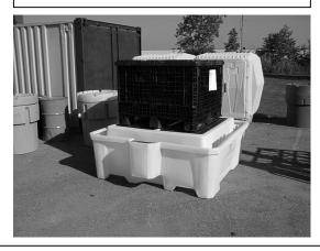
5.) The maximum load is 8,000 lb (3,628 kg). The load must be centered on the pedestal.
